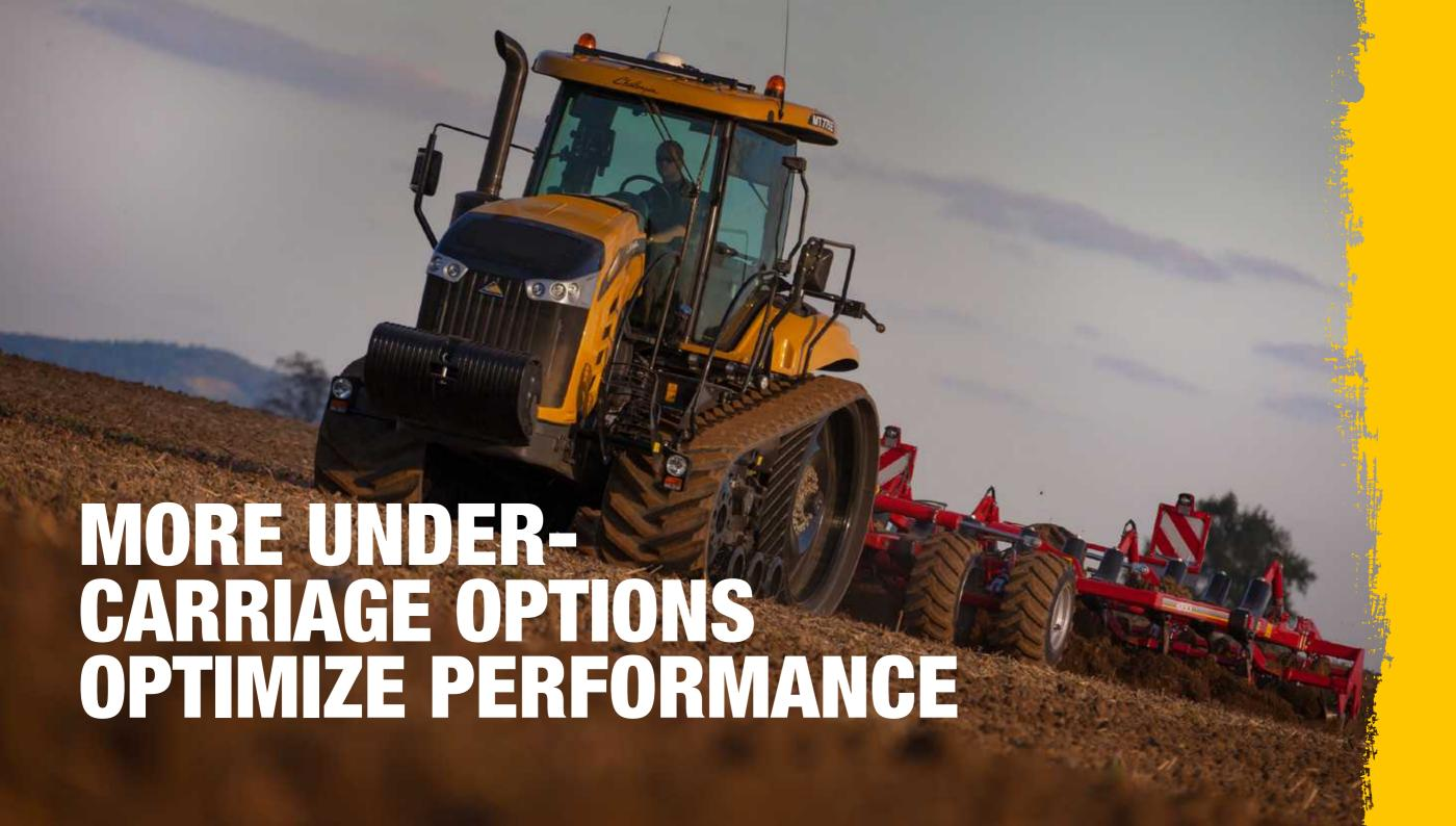
The Challenger MT700E Series tractors offer more Mobil-Trac System options than ever before allowing you to tailor your tractor to your applications. Belts are available in six widths and in three types. Only tractor across the industry Challenger MT700E Series offers three idler, mid-wheel and driver widths. Two infinitely adjustable gauge ranges are available to match your applications, according local road legislation.
