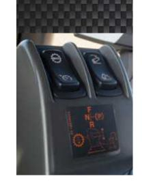
The intuitive One-Touch headland management system gives you the power to initiate several tractor and implement functions at the same time with the simple push of a button. Easy to operate, the One-Touch management system uses the Intellitronics network to record and execute functions such as transmission shifting, throttle, 3-pt linkage position, PTO status, implement lift and lower, and Auto-Guide.
