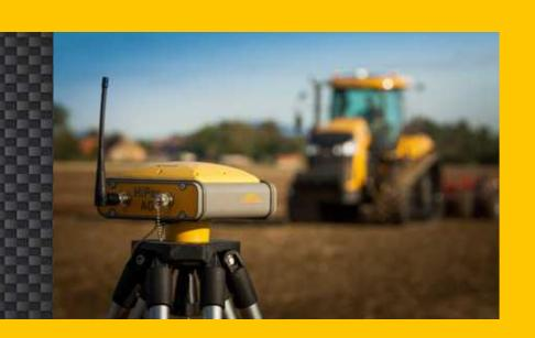
The flexibility to perform precision applications like bedding, planting and tillage are built right into the Auto-Guide satellite navigation system. The GPS receiver sends location information to the implement variable rate controllers via the Intellitronics and ISO11783 networks.
