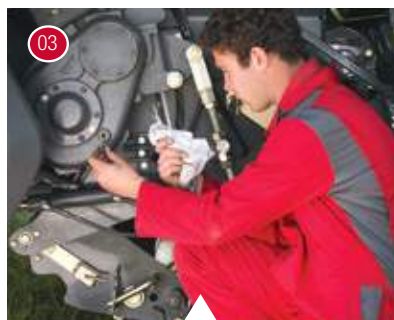
03 Checking the cutter gearbox oil level.
