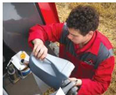
Refilling the automatic chain oiler.
