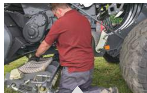
Ample accessibility offering straightforward knife removal
