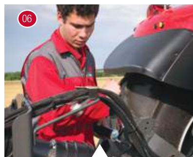
06 Greasing the PTO shaft.
