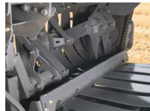
The Packer tines ensure even feed into the pre-compression chamber.
