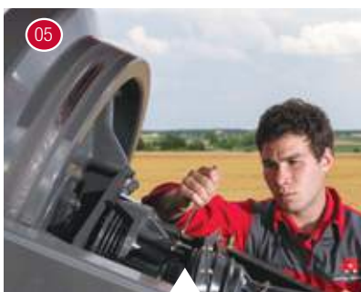
05 Adjusting the flywheel slip clutch.
