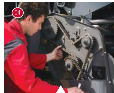
04 Checking the pick-up chain tensions.
